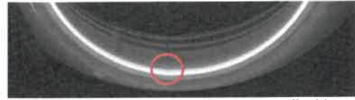
Figure 13: Process image classified “mono” with growth line visible in the meniscus region
