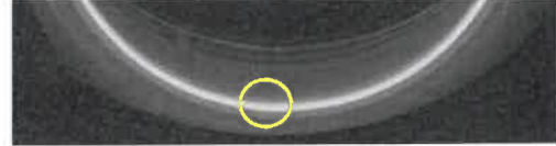
Figure 14: Process image classified “sl” with growth line outside the meniscus region
