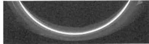
Figure 15: Process image classified “sl” with absence of growth line
