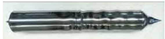
Figure 12: Crystal with a deviation from the cylindrical shape (spiral growth).
