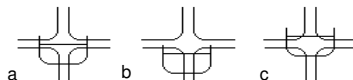
CUSP plane configurations relative to the melt level: a) CUSP plane on melt level, b) CUSP plane in the growing crystal, c) CUSP plane in the melt
