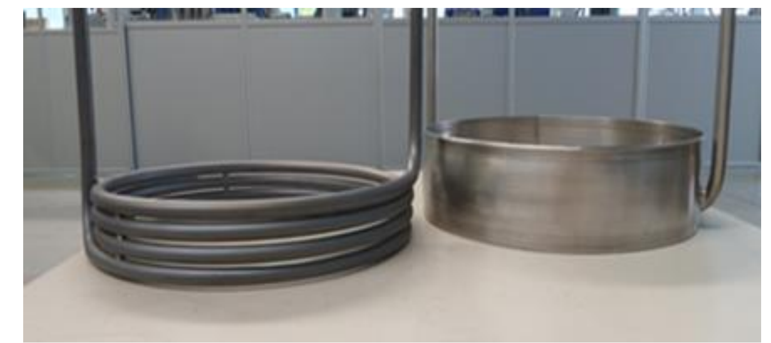
Cooling container with a spiral shape and a cylindrical shape with different surface emissivities.
