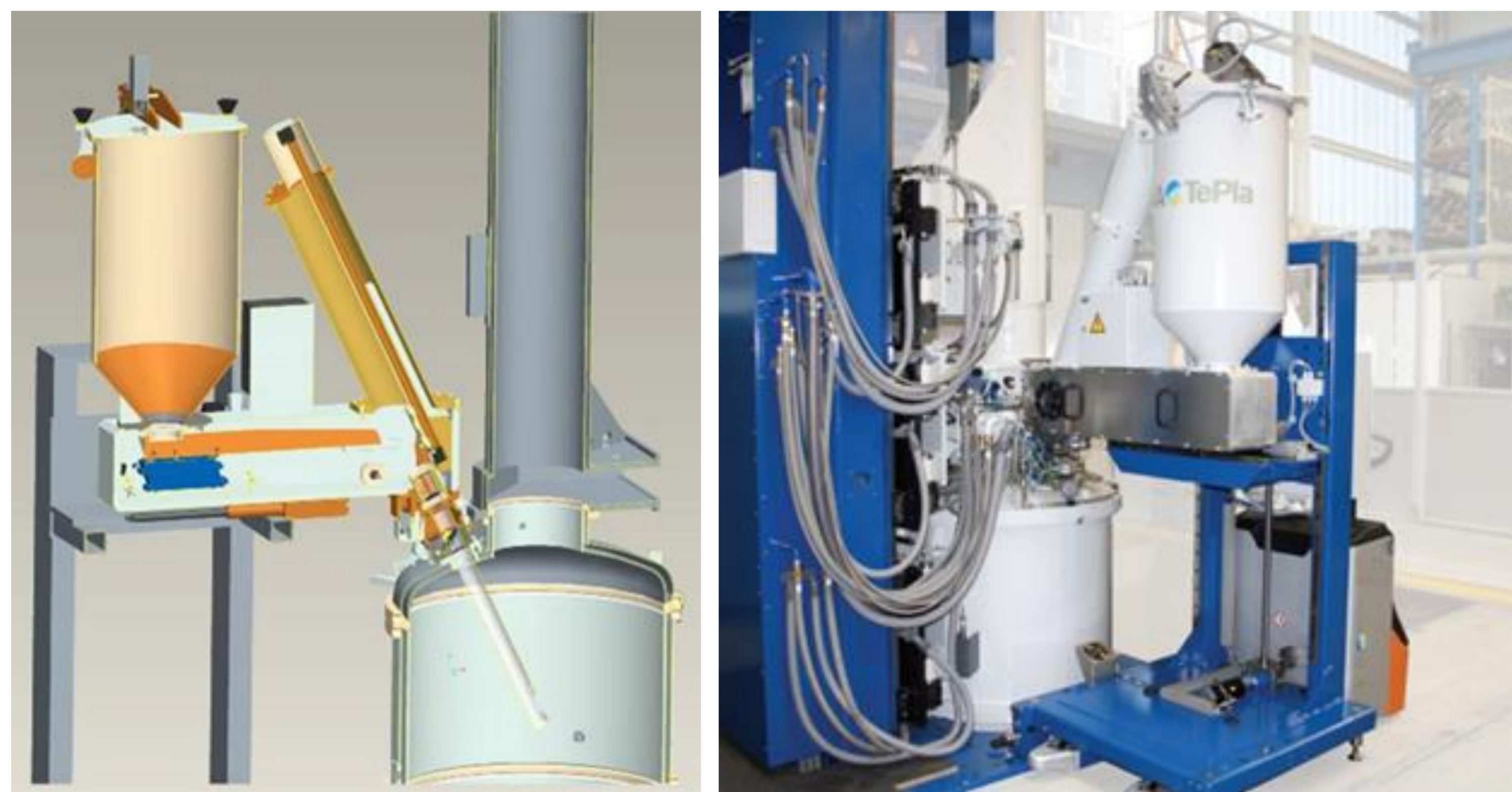
Mobile Recharge System (MRS) from PVA Crystal Growing Systems GmbH
