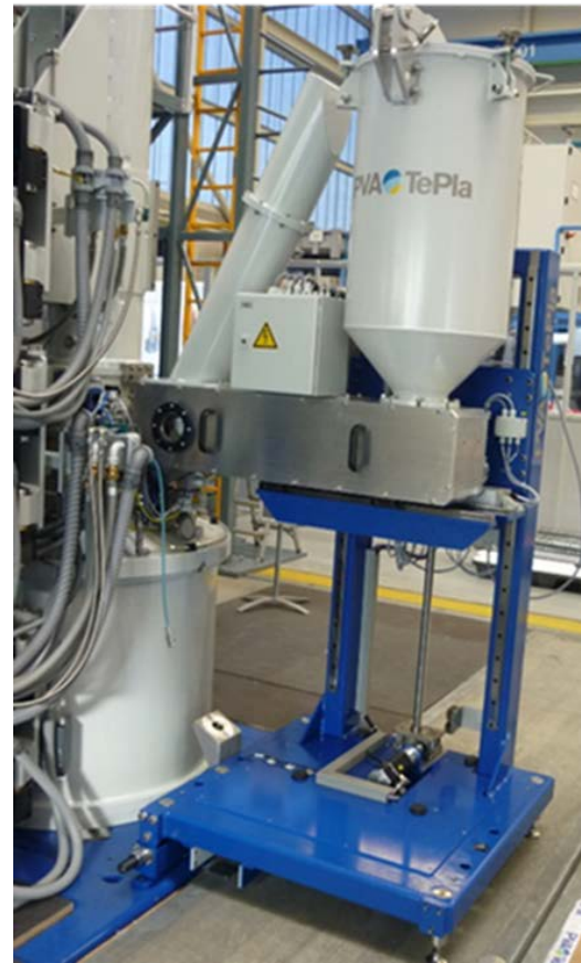
Figure 3: Mobile recharge system docked on a Cz-puller
