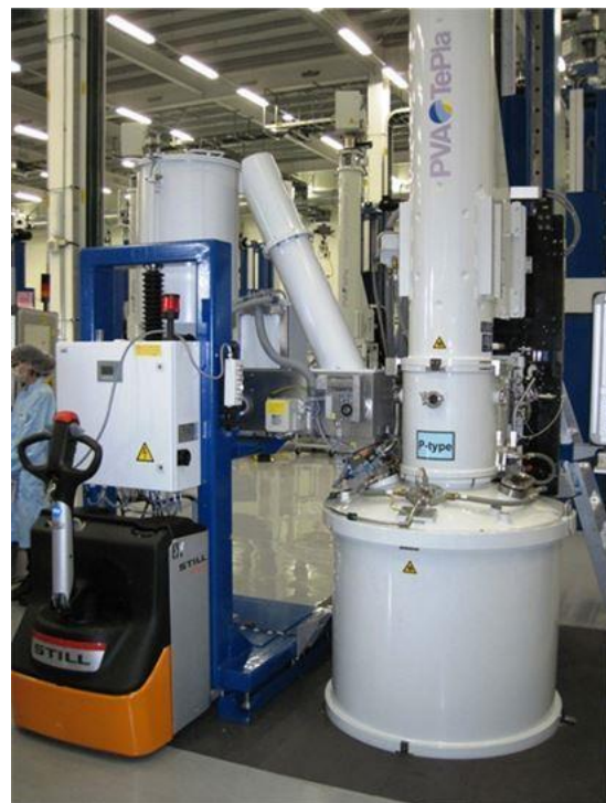
Figure 4: Mobile Recharge System docked on Cz-puller
