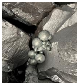
Figure 4: Ga beads surrounded by silicon chunks
