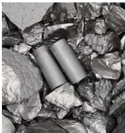
Figure 3: Ga embedded in a closed silicon container surrounded by silicon chunks
